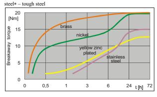
The graph below shows the relative increase in breakaway torque developed with time using activator A. Developed on M10 medium bolts and nuts. Tested according to ISO 10964.
