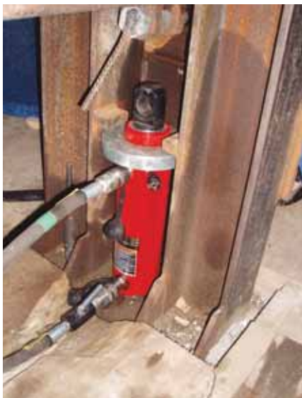
HD cylinders can be used in pushing and pulling applications. In this photo, we see a HD2506 HD cylinder set up for a pull application using a plunger clevis cylinder accessory
